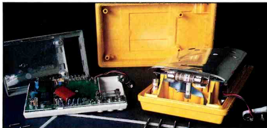
Note the difference in size and mechanical ruggedness of the heavy duty DMM (left), the professional DMM (middle), and the low cost DMM at the right.
